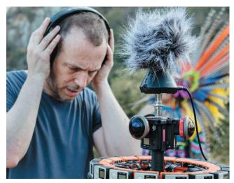
Monitor your audio live in stereo binaural or use the H3-VR's onboard Ambisonics Decoding to simulate your recorded 360-experience during playback.
